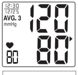
3. Press the **M** button again. The LCD will display the latest measurement. Press **M** or **8** buttons to scroll through all stored measurements.
